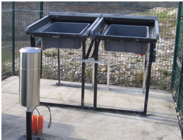
Figure 3. Two compartments sampler for atmospheric dry fallout and rain water in Chassieu, with the rain gauge at the forefront (photo AD).
